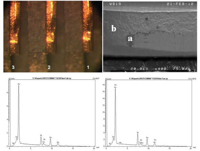
Figures 2-5 Clockwise from top left: Optical photo of contacts, SEM image, EDX charts (areas a and b)
