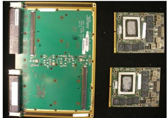
Figure 1. Photo of disassembled vibration test vehicle (MXM heat sinks and other metalwork removed)
